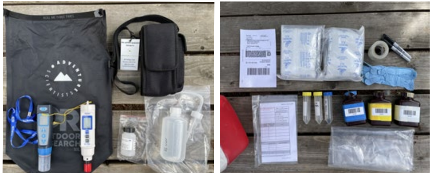
EQUIPMENT PROVIDED TO VOLUNTEERS TO CONDUCT FIELD MEASUREMENTS (LEFT) AND COLLECT GRAB SAMPLES (RIGHT).
