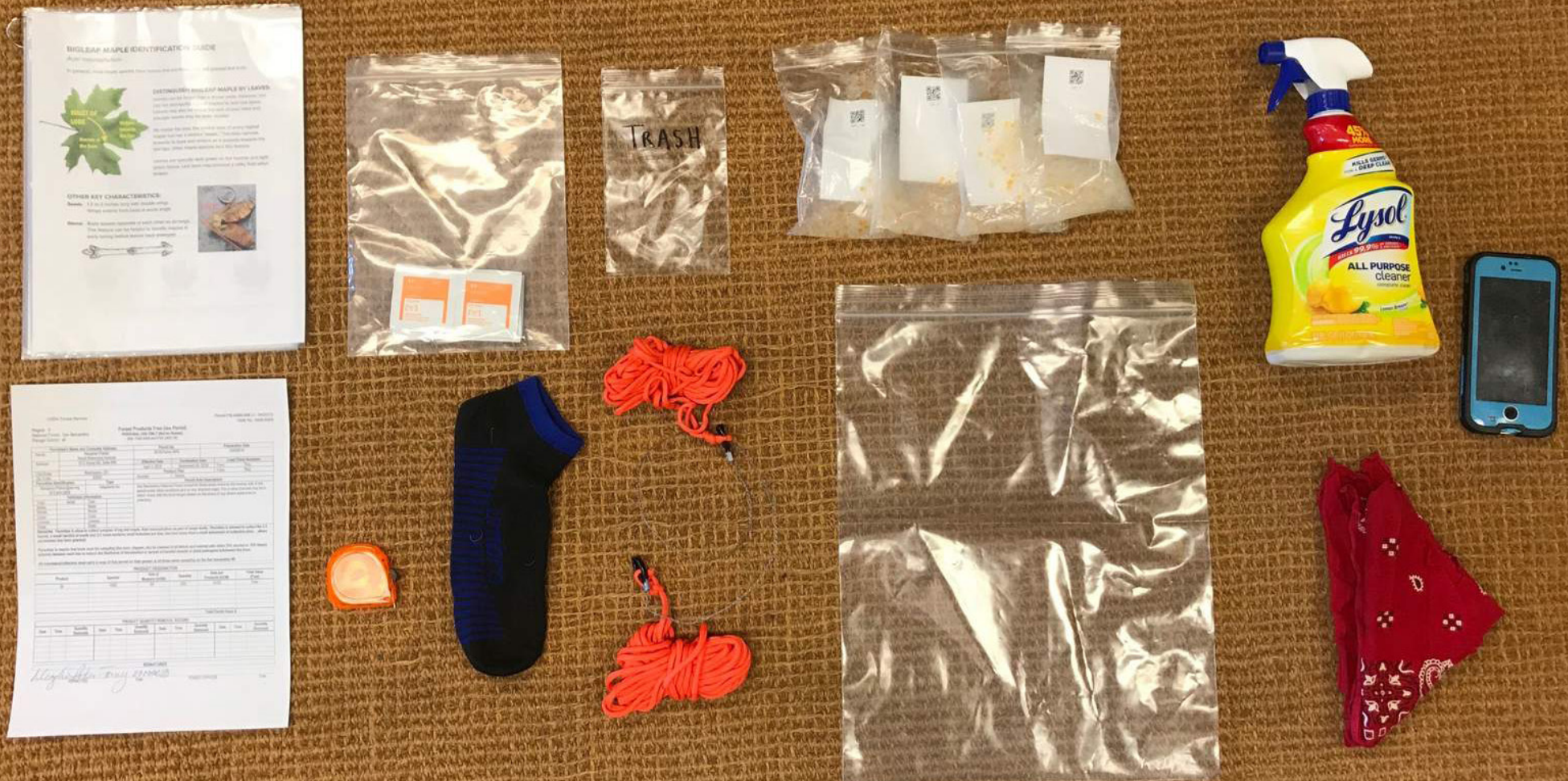
LEAF CREW EQUIPMENT CONSISTED OF SAMPLING PACKETS, A SAW-TOSS TOOL, ALCOHOL WIPES, AND A LIGHTWEIGHT MEASURING TAPE
