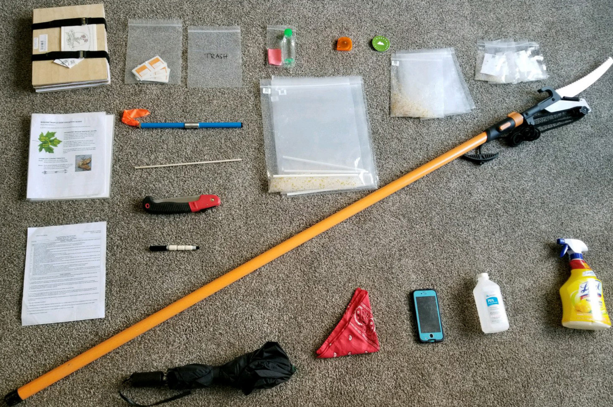
WOOD CREW EQUIPMENT CONSISTED OF SAMPLING PACKETS, A PLANT PRESS, AN INCREMENT BORER, A POLE SAW, A HANDSAW, A CLEANING KIT, AND A LIGHTWEIGHT MEASURING TAPE.
